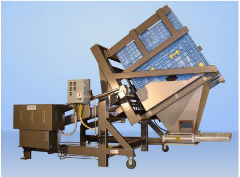
floor level, and provide a “sealed discharge” of the containers under a 10’ ceiling height. The dumpers also needed to be moveable, to allow for regular wash down of the equipment and process area.
