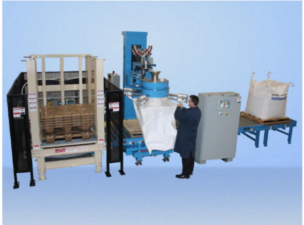
full pallet handling capabilities, including the ability to dispense three (3) different types and sizes of pallets (2-way, 4-way, or nestable OSB) into the filler unit, and automatically discharge the filled containers on pallets for forklift removal. The equipment needed to be reliable, PLC controlled, and easy to operate from floor level.
